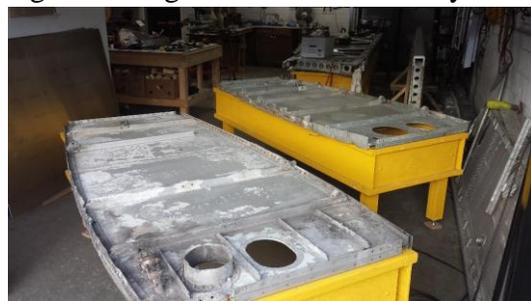
So this is Phase 3a (rebuilding and replacing wing ribs). THEN we will move on to Phase 3b which is rebuilding and restoring the Halifax REAR spar.
