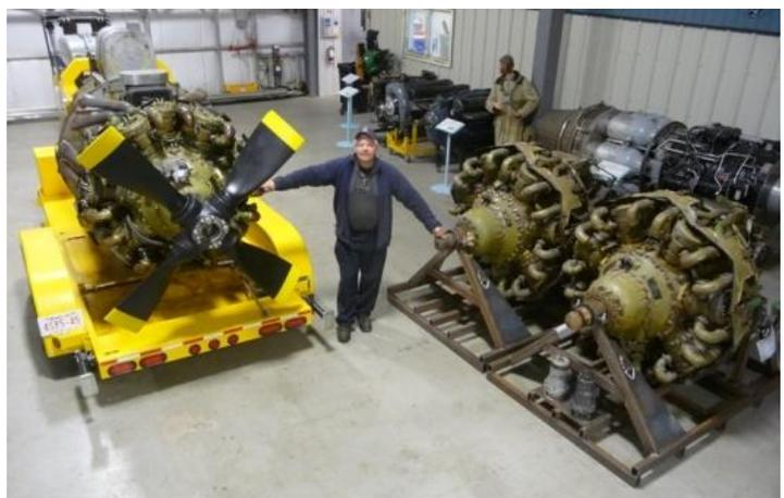
So once we have scavenged all the parts we need off the donor Hercules we can get into working on #2, #3, and #4. These Hercs will be refurbished and go along side the running Hercules #1 we have on the yellow airshow display trailer which is also our engine run test-bed.
