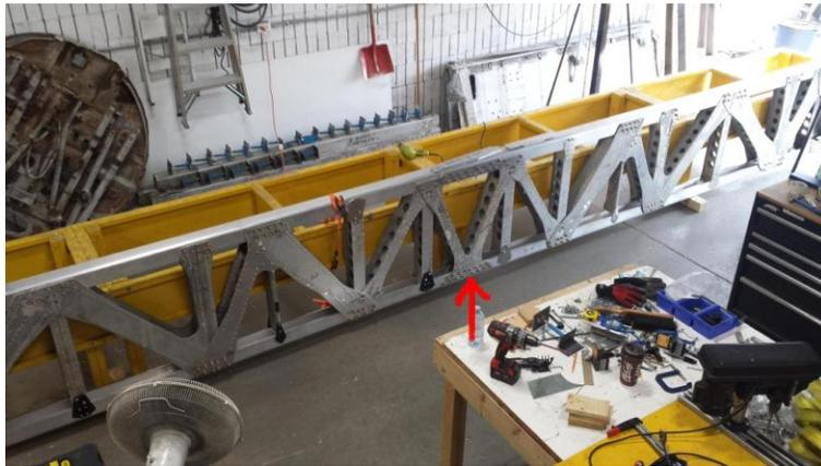
Now we are moving on to Phase 3a which is the 10 wings ribs which attach to the face of the main spar and extend back towards the rear spar. See the photo (below) of the center-section of Halifax NA337 being rebuilt in Trenton. The RED arrow is the main spar face down and the GREEN arrow is one wing rib rebuilt and being attached. See next to the NA337 photo a pic of 2 of our wing ribs being readied for rebuild by Knox Tech.
